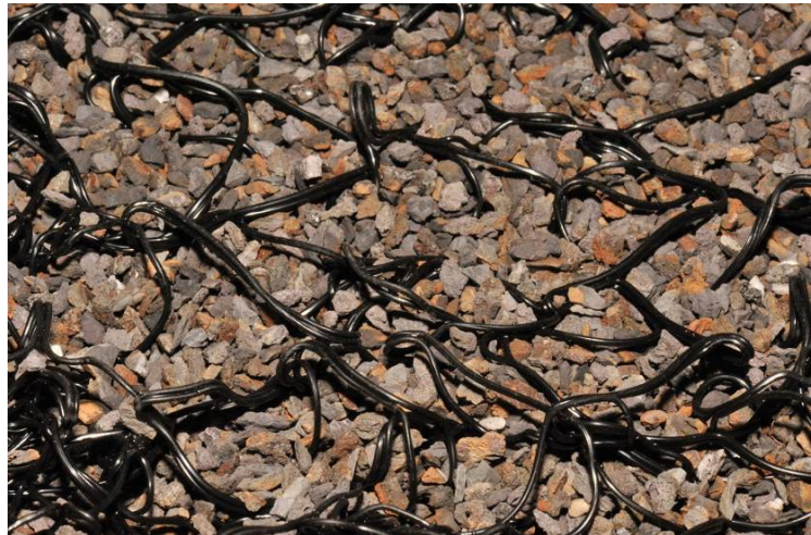
Figure 20...21: Claw mat placed on the slope (unfilled) and a filled with crushed grains of size 1 to 3 mm
