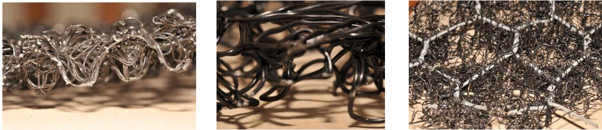
Figure 1...3: Claw mats of polypropylene as mazy laid structure and in combination with a grid net
